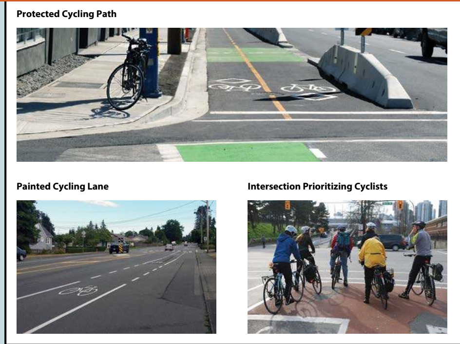
Figure 4.12 Sample of Infrastructure Measures to Increase Cyclist Safety
